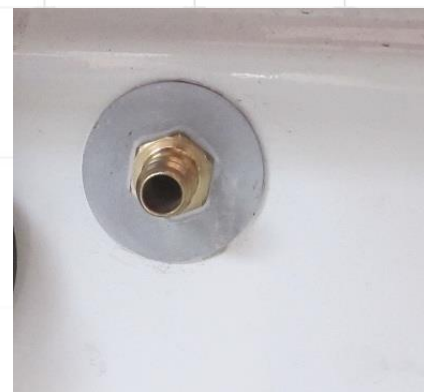
Photo. 8a) Instantaneous coupling of compressed air supercharging
